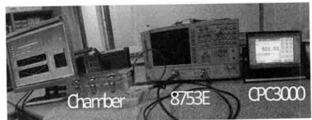
Fig. 6. Sensor characterization system. System is composed of vacuum chamber, network analyzer (HP 8753E) and precision pressure regulator (CPC3000)
