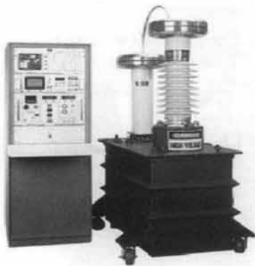
Fig. 2. Experimental equipment of partial discharge.
