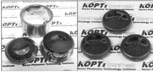
Fig. 11. Mold and molded lens fabricated in this study.
