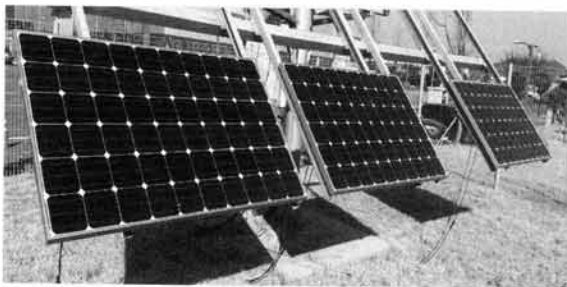
Fig. 3. Field test with different types PV modules with conventional soldering (SR) and low-temperature CF bonding (CF-LCR, CF-PFR).
