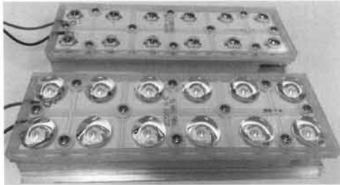
Fig. 6. LED 60°, 120° lens heatsink prototype.
