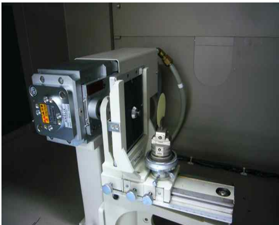
Fig. 6. Rigaku D/Max 2200 powder X-ray diffractometer.
