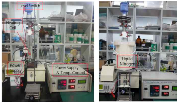
Fig. 11. Test setup to evaluate the temperature characteristics. (a) high, (b) low temperature.
