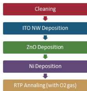
Fig. 1. Fabrication steps of ITO NWs-embedded n-type ZnO/p-type NiO heterojunction photoelectric device.
