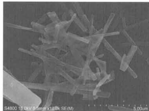
Fig. 4. The FE-SEM image of the synthesized sample at the condition of \text{Na}_2\text{CO}_3 : \text{TiO}_2 : \text{NaCl} = 1 : 6 : 35 by mol.
