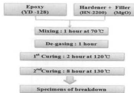
Fig. 2. Block diagram of specimens manufacturing process.
