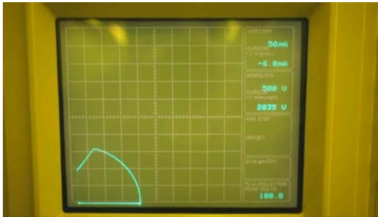
Fig. 11. The measured data of super junction IGBT with super junction field rings.
