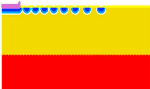
Fig. 1. The structure of field rings for conventional NPT IGBT.
