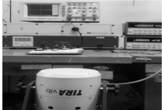
Fig. 6. Measuring setup for applying tensions to the harvester.
