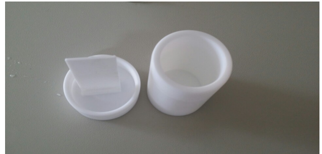
Fig. 1. Photograph of the laboratory-made reactor for the hydrothermal growing of ZnO nanorods.
