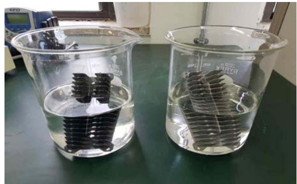
Fig. 4. Salt corrosion testing of heat sink.
