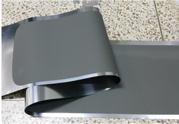
Fig. 4. FeS 2 thin film cathode sheets with about 180 \mu\text{m} thickness and 230 mm in width.
