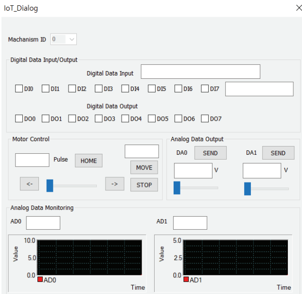
Fig. 12. GUI implementation for control and monitoring of mechanism modules.
