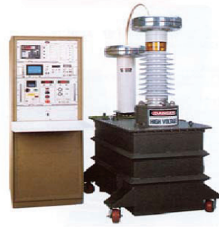
Fig. 1. Experimental equipment of partial discharge.
