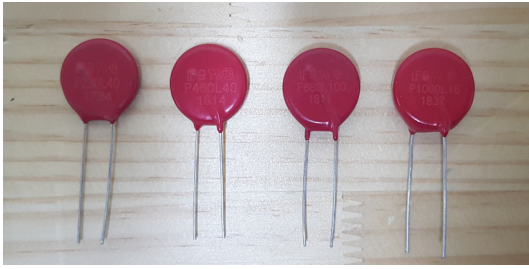
Fig. 4. The varistors used in test.
