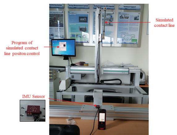
Fig. 4. Configuration of simulated contact line detector included imu sensor.
