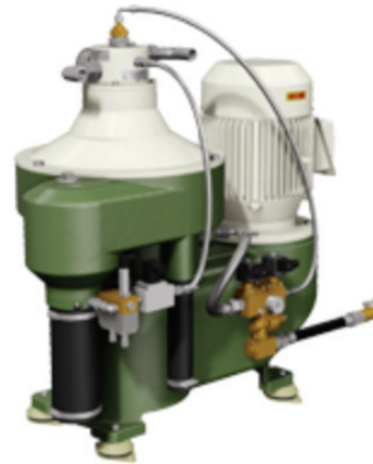
Fig. 4. Liauid compound separator (model: SO-300D).
