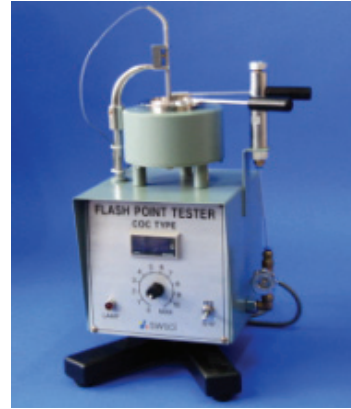
Fig. 3. COC flash-point tester.
