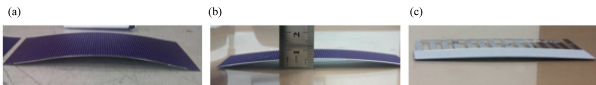
Fig. 5. Bending characteristics of divided cell strips: (a) type-1, (b) type-2, and (c) type-3.
