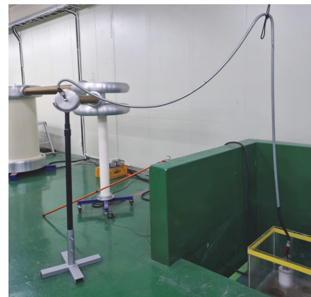
Fig. 8. Photograph of voltage conditioning.
