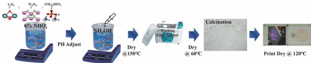
Fig. 1. Process flow chart of YPO_4:Pr^{3+} synthesis and DBD plasma device.
